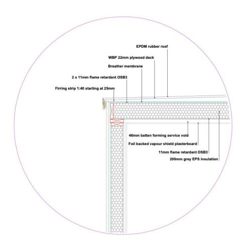
Complete roof build up U-value: 0.18 W/(m2K)
