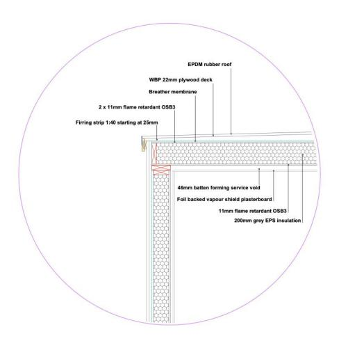
Complete roof build up U-value: 0.18 W/(m2K)
